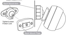
Note: The Back-Mount Arm may be locked in various angles by turning the Friction Lock clockwise and counter-clockwise to tighten or loosen (respectively) the angle of the arm.
