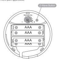
Troubleshooting: If the Multisensor was not successfully paired into any Z-Wave network, the LED which is on the Multisensor will blink when pressing the Z-Wave Button. If the Multisensor was successfully paired into a Z-Wave network, the LED will stay solid for a few seconds when pressing the Z-Wave Button.
